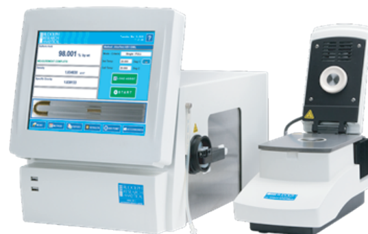
Fig. 3 Setup for determining high concentrations of H 2 SO 4 . Showing manual injection
